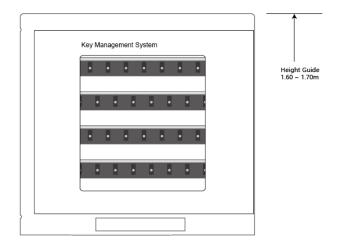
Step 2. Mark and drill 6 fixing holes and attach the wall bracket to the wall using the appropriate fixings.
