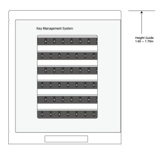
Step 2. Mark and drill 6 fixing holes and attach the wall bracket to the wall using the appropriate fixings.
